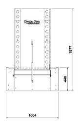
Electrical 200-240Vac Single Phase Max Current 20 Amps (With Fans) Fuse at 20 Amps 2.5mm<sup>2</sup> Minimum Cable size recommended
