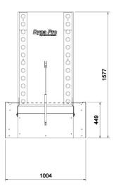
Electrical 190-240Vac Single Phase Max Current 20 Amps (With Fans) Fuse at 20 Amps 2.5mm<sup>2</sup> Minimum Cable size recommended
