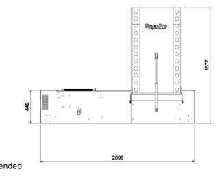
Electrical 190-240V ac Single Phase Max Current 20 Amps Fuse at 32 Amps 6mm<sup>2</sup> Minimum Cable size recommended
